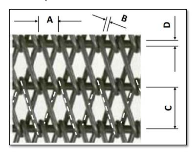
**NOTE:** When measuring pitches A & C, it is best practice to measure over 10 pitches and then divide by 10 to obtain the average pitch.
